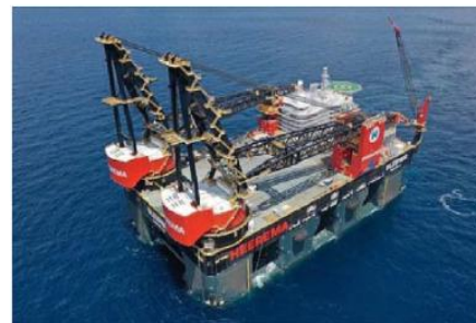
f) Semisubmersible construction vessel
