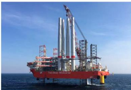
e) Purpose-built jackup vessel
